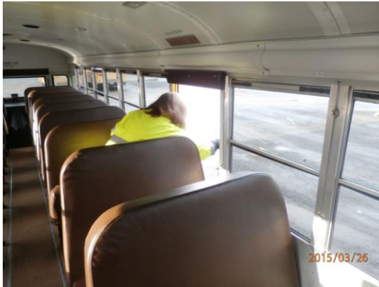
Opening / Closing Escape Hatches on the side and rear of bus for Pre-Trip Inspection.
