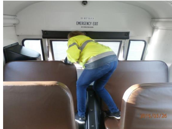
Opening / Closing Escape Hatches on the side and rear of bus for Pre-Trip Inspection.
