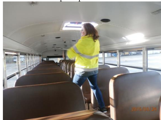
Opening / Closing Escape Hatch for Pre-Trip Inspection.
