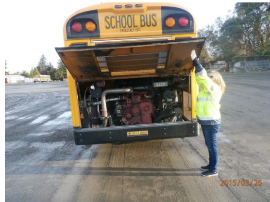
Opening/Closing Re-Compartment for Pre-Trip Inspection.
