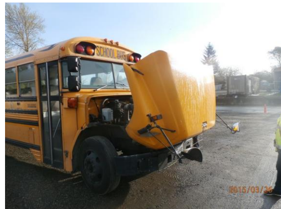
Pulling open hood for Pre-Trip Inspection.
