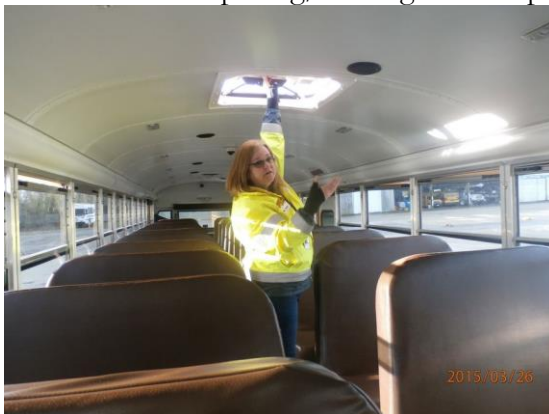
Opening / Closing Escape Hatch for Pre-Trip Inspection.
